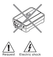
Please check the use voltage and current for the DC-only products and use the appropriate rectifier.
