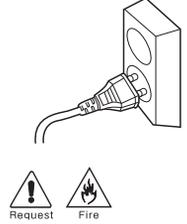
Please hold the plug tightly when unplugging the power cable (a part of the copper wire may be disconnected if the grabbing is only made on the cord when pulling out the cable).
